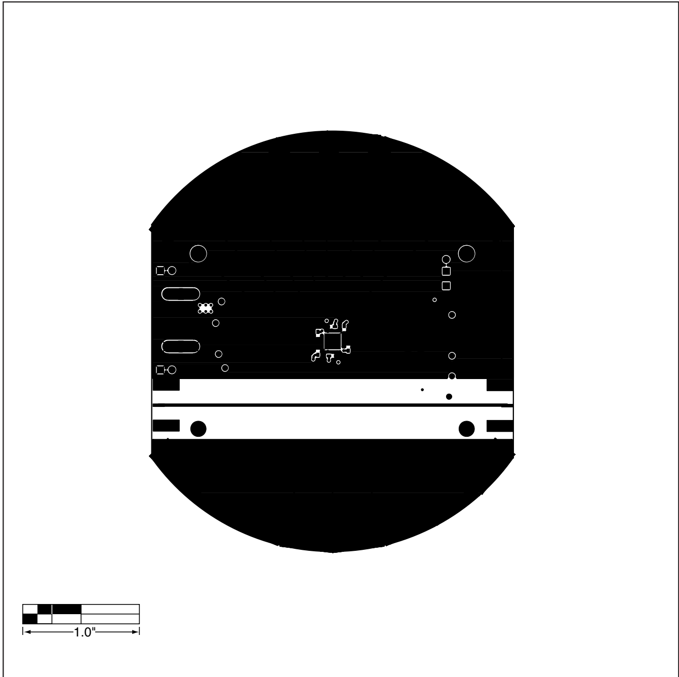
Figure 7. MAX3980/MAX3981 EV Kit PC Board Layout—Solder Side
