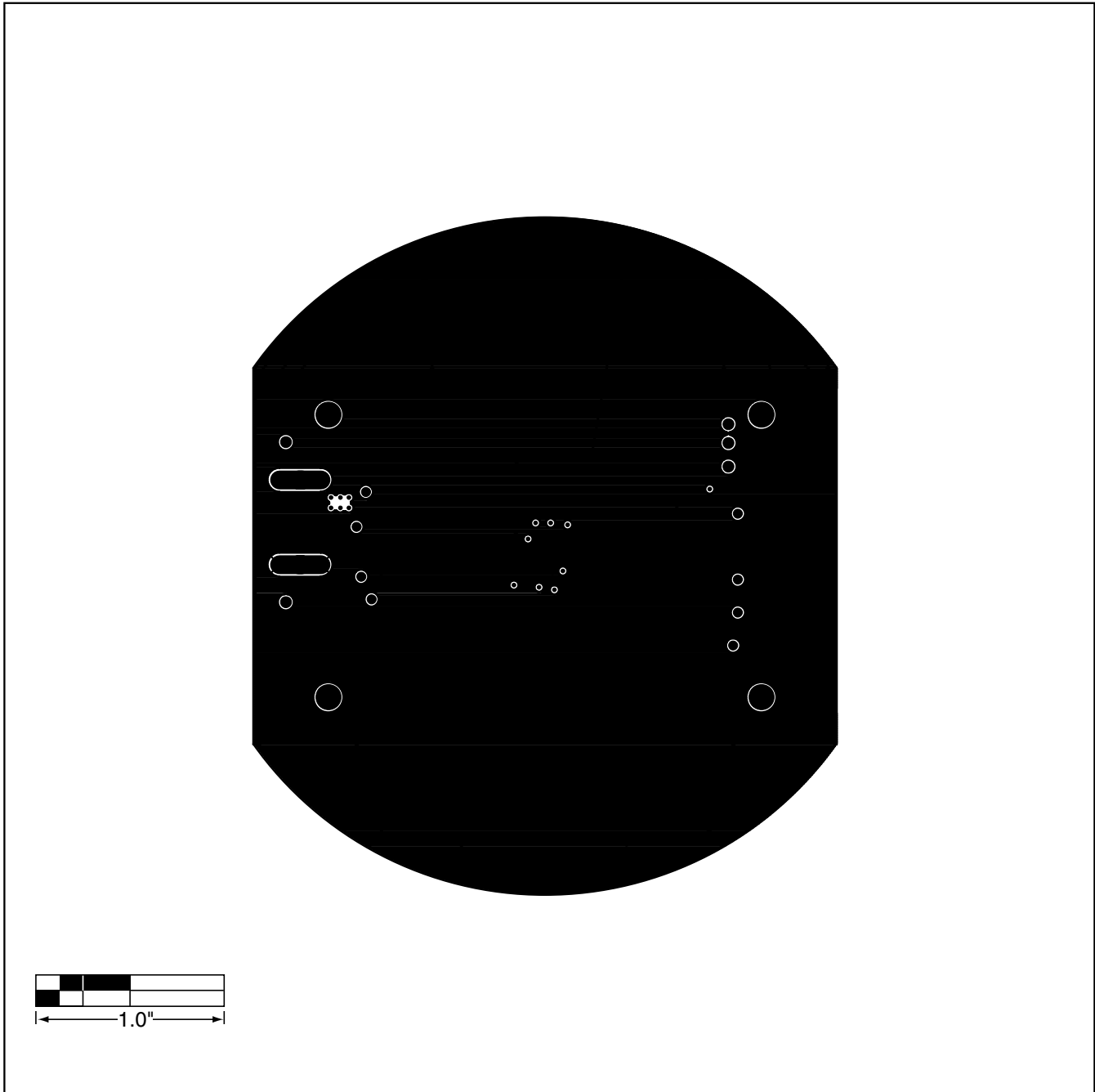
Figure 5. MAX3980/MAX3981 EV Kit PC Board Layout—Ground Plane
